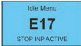
If an error occurs, it is displayed in a window occupying the entire display similar to the example shown at left. Find the error code in the tables included in this chapter to determine the cause and corrective action.
